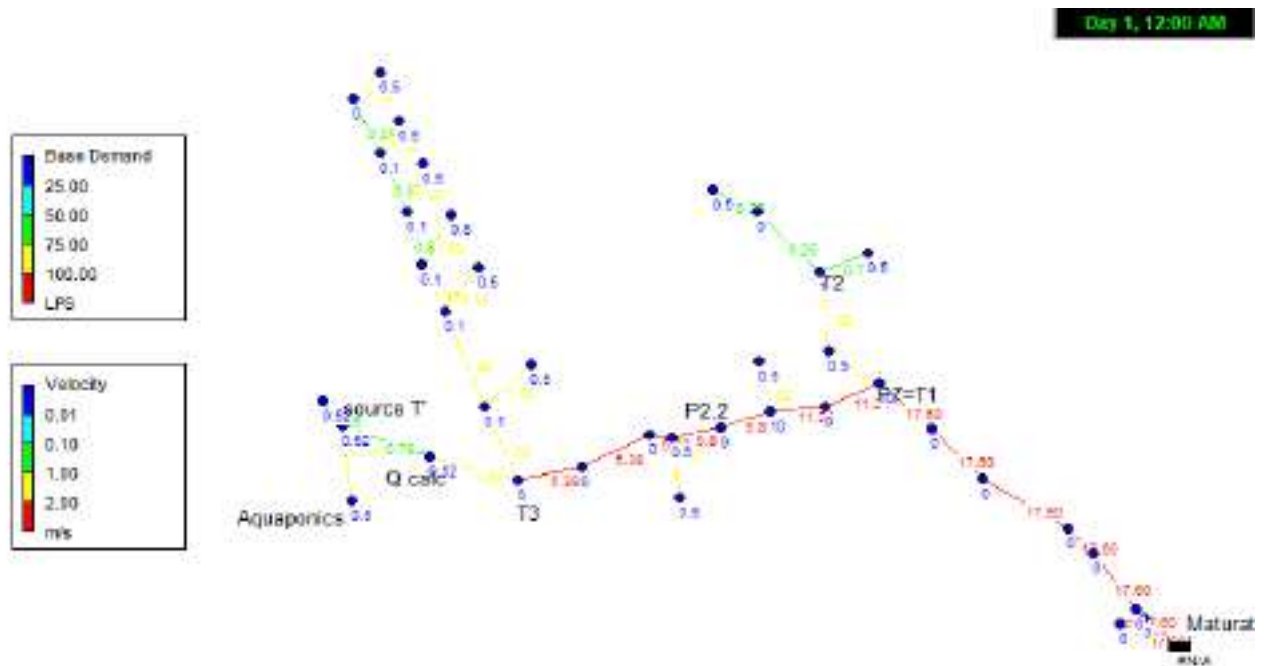
Figure 6: simulation of the irrigation pipelines established in GDA Sidi Amor. Source: EPANET 2.0
